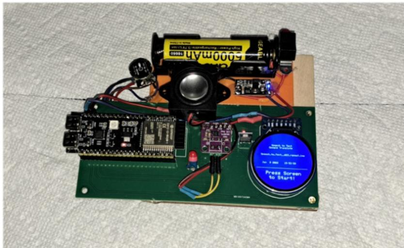
Both of these have the same software and communicate to the same A-I website. The difference is how much smaller and neater the bottom one is. The smaller speaker is the silver button. All those jumpers are replaced by the green circuit board underneath the ESP32 microcontroller. It is unbelievable how cheap and easy it is to replace the jumper board with a circuit board. There is some effort involved in learning how to design the
