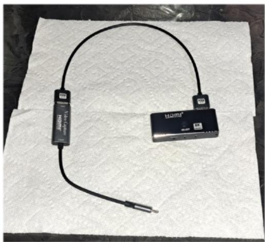
USB output. Larry uses it to connect his new Icom IC-7300MK2 transceiver to a 15-inch video monitor or his computer.
