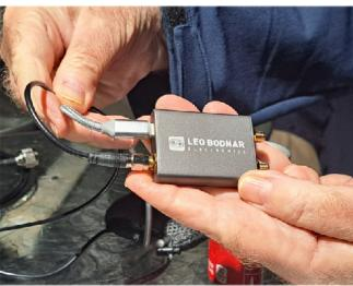
Below, Larry is holding an 8-way GPS antenna splitter.
