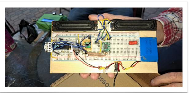
The device between the ESP8266 and the receiver board is an IR receiver for the remote control. He did not have to buy one for this project, he had one in his junk box. It controls the radio chip.
