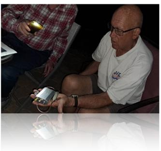
Here's the RTL-SDR that **John Mock** brought. It was an older version of what Ray Rounds brought. The dongle is a Nooelec Nesdr Smart XTR. It attaches to a Nooelec "Ham It Up" upconverter so you can listen to the ham bands. The reason is that the dongle only goes down to 55MHz (instead of Larry's 0.5 MHz)
