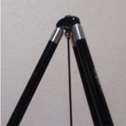
The magnet is connected to graphite rod I had, and the pivot was a steel ball that was stuck to a disk magnet that held itself onto the bottom of the tripod. I couldn't believe my luck. The pivot mechanism went together in less than a minute. The motion is a random swinging that can go on for hours or just a few seconds. So it's not at all perpetual, but it is much more amusing. The swings are so random both in direction and in amount.
