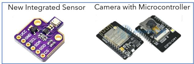
Both devices are about ten dollars each !! The camera has a computer, WiFi, microSD recorder and storage for dozens of HD imagery.
