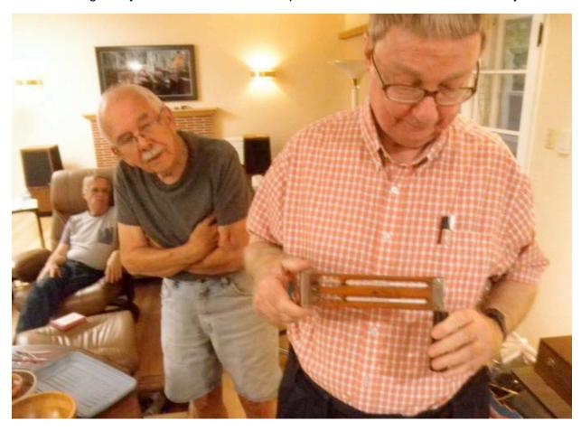
The one he's holding is a "sling" psychrometer. The handle in his left hand allows the bulb end of the two thermometers to whirl around in the air. He had one other sling psychrometer and two of the type which use a wind up spring powered fan to draw air past the thermometers.
