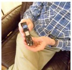
The glass thing he's holding was made for him by a glass blower friend of his. Notice that it is a flattened bubble shape. It is evacuated with a blob of ultra-pure mercury that can slide around by moving the hand. With the lights out it was easy to see an orange glow from inside, on the surface of the mercury. Because the mercury has to be moving it wasn't easy to see any detail.
