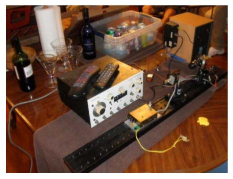
It was only a distance of a foot or so, but it showed his source and detector working in the AM mode. Although it passed throug an RF driven Bragg Cell, he was unable to demonstrate beam steering. Just for fun he demonstrated what a TV remote sounds like when decoded with his AM detector.
